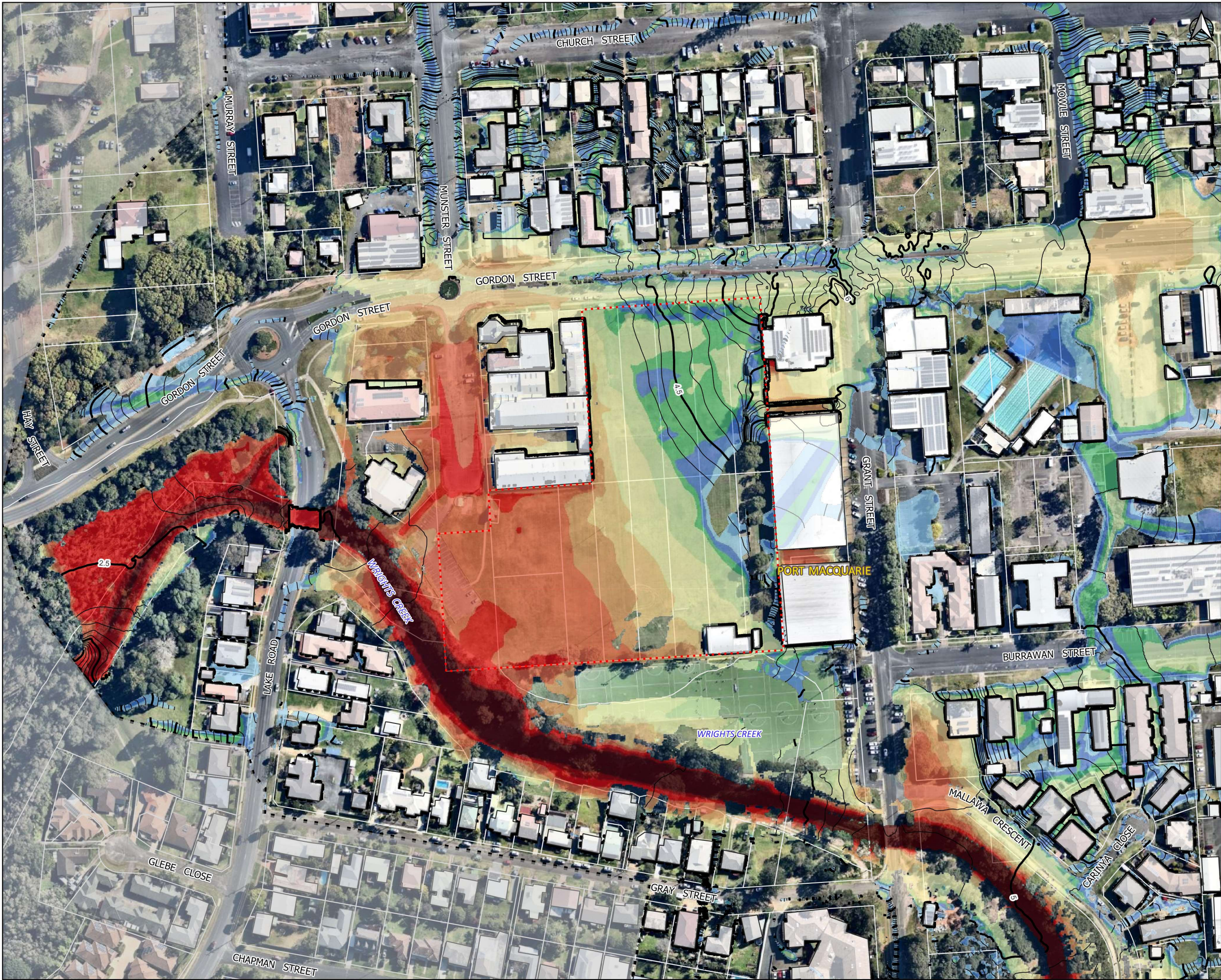
Figure B6 [A] Existing Case 1 in 200 AEP Flood Depth and Elevation Envelope of Local and Regional Flood Events
