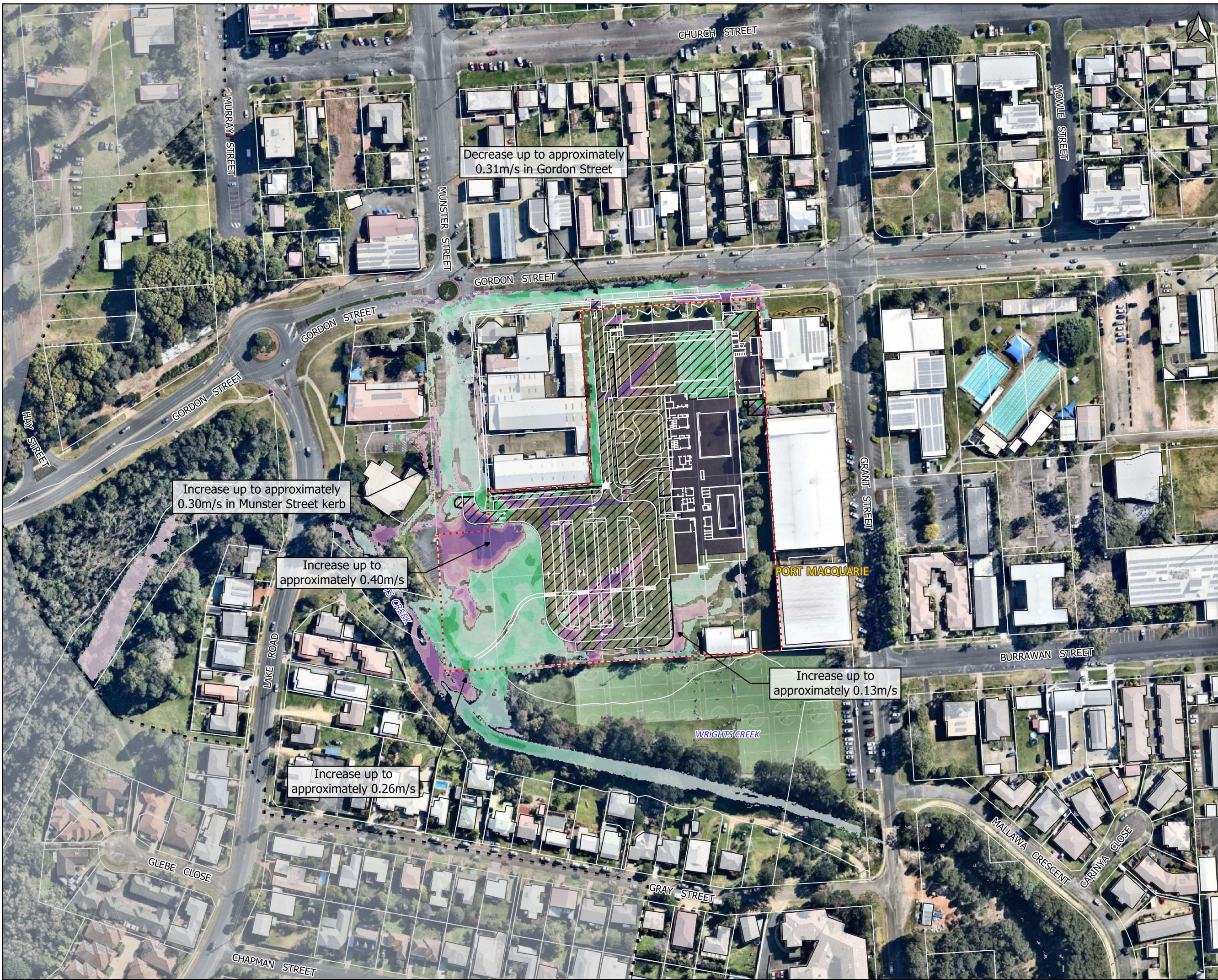
Figure D2 [A] Pre to Post Comparison 10% AEP Flood Velocity Local Catchment w/ Neap Tide Tailwater
