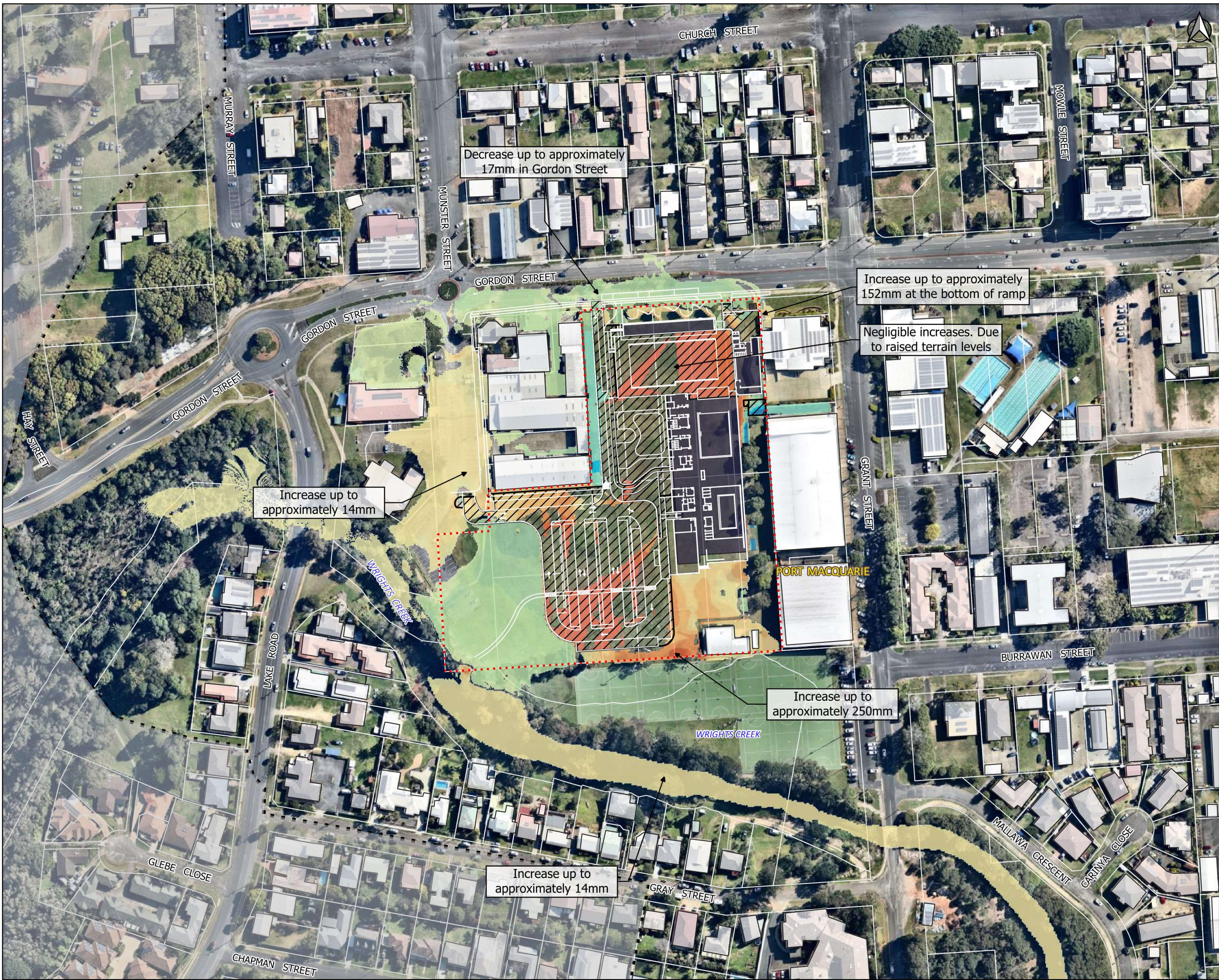
Figure D5 [A] Pre to Post Comparison 1% AEP Flood Elevation Local Catchment w/ Neap Tide Tailwater
