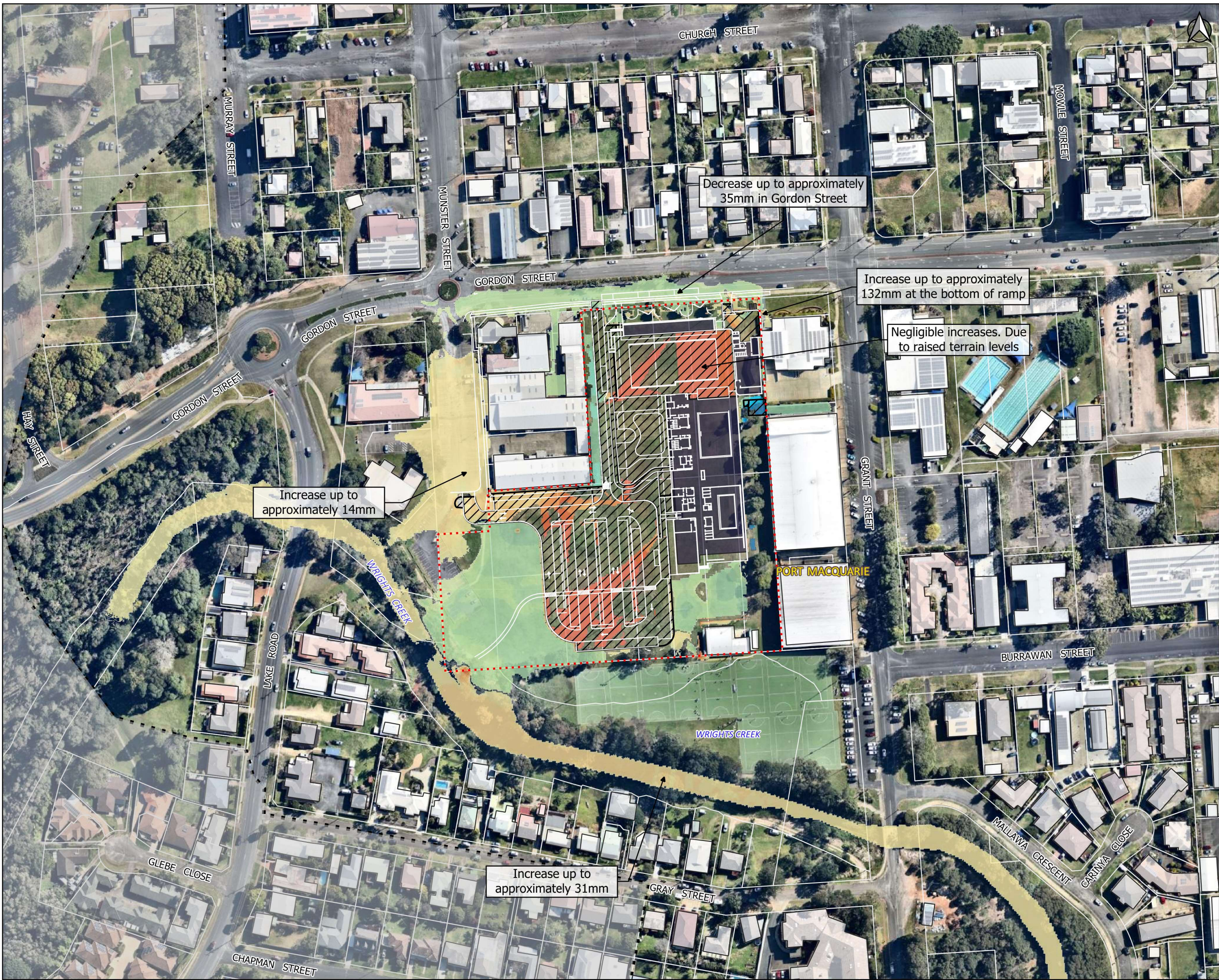
Figure D3 [A] Pre to Post Comparison 5% AEP Flood Elevation Local Catchment w/ Neap Tide Tailwater
