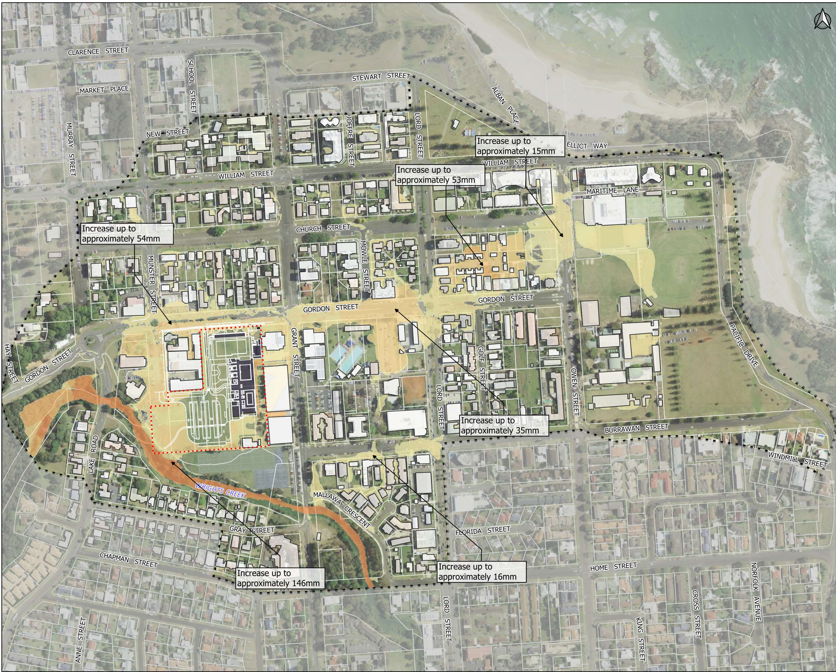
Figure E1 [A] Climate Change Scenario 1 in 200 AEP minus 1% AEP Flood Depth Local Catchment w/ Neap Tide Tailwater
