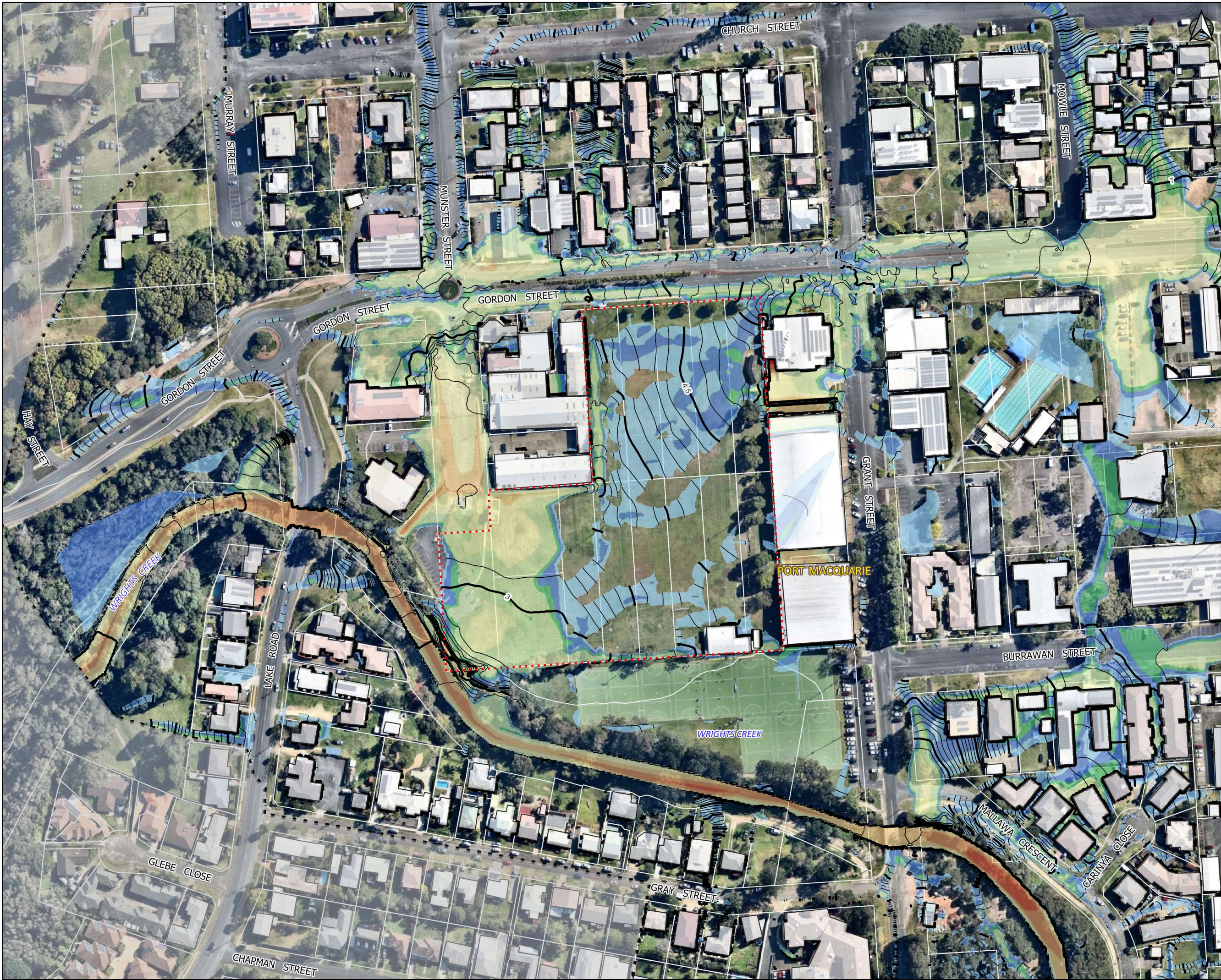
Figure B1 [A] Existing Case 10% AEP Flood Depth and Elevation Local Catchment w/ Neap Tide Tailwater
