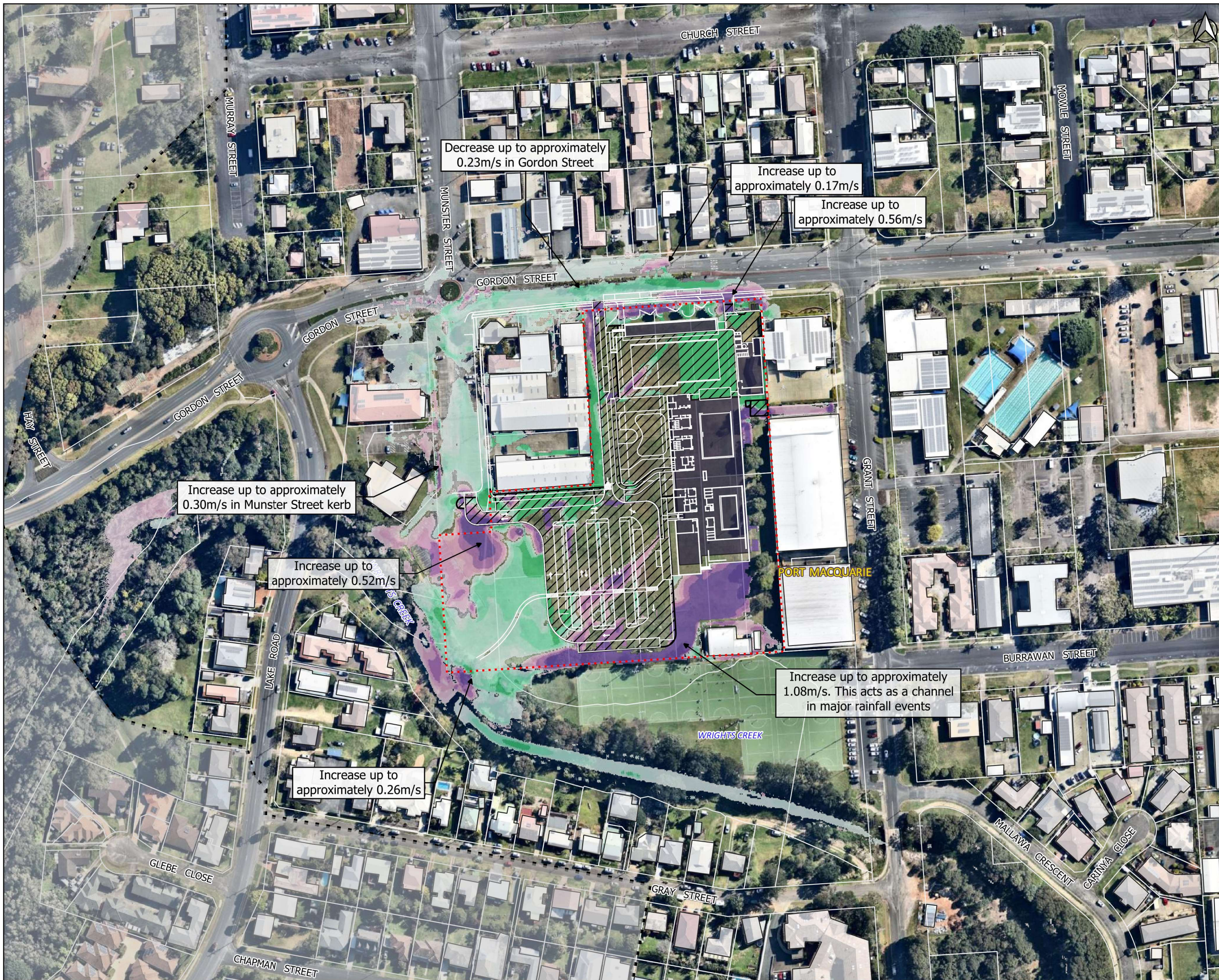
Figure D6 [A] Pre to Post Comparison 1% AEP Flood Velocity Local Catchment w/ Neap Tide Tailwater
