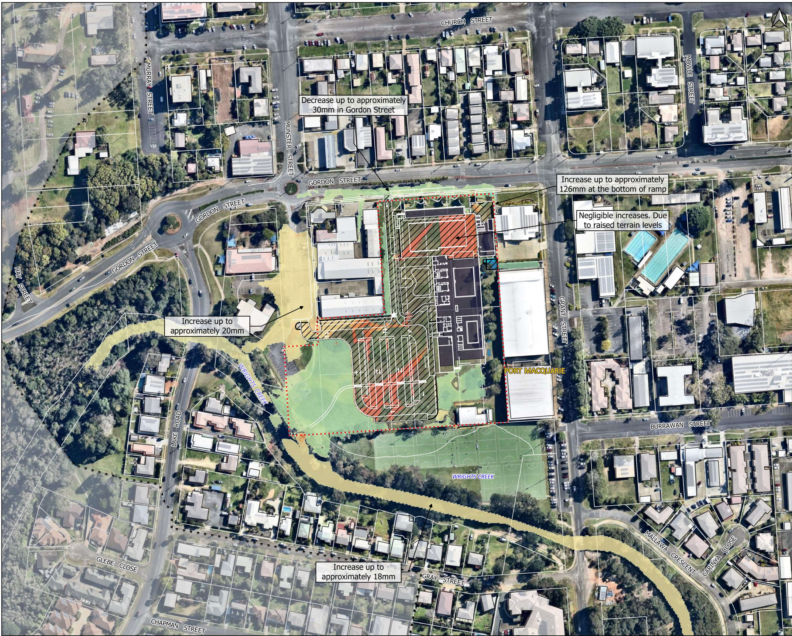
Figure D1 [A] Pre to Post Comparison 10% AEP Flood Elevation Local Catchment w/ Neap Tide Tailwater
