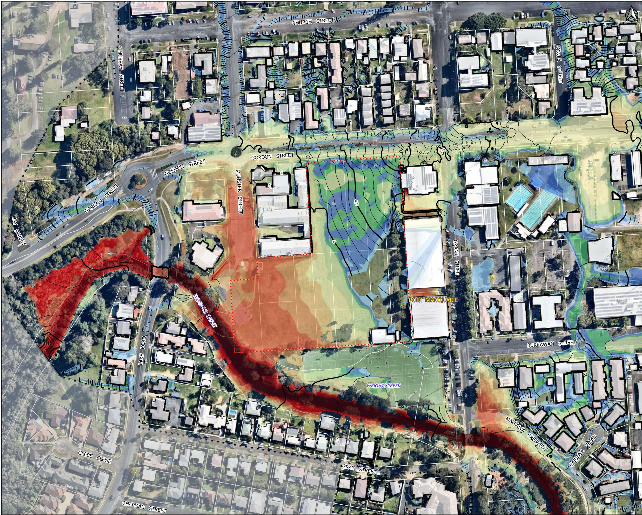
Figure B4 [A] Existing Case 1% AEP Flood Depth and Elevation Envelope of Local and Regional Flood Events
