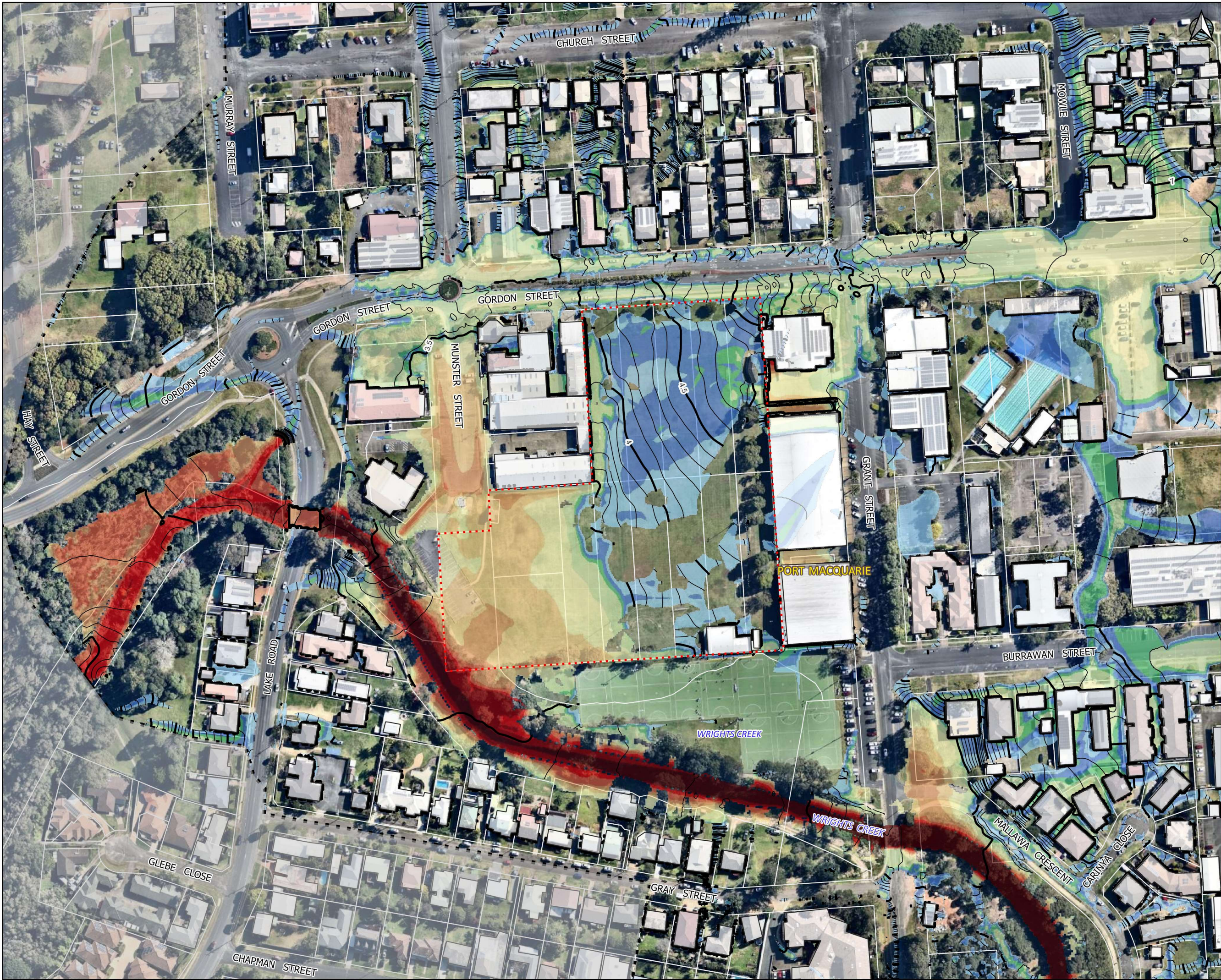
Figure B2 [A] Existing Case 5% AEP Flood Depth and Elevation Envelope of Local and Regional Flood Events
