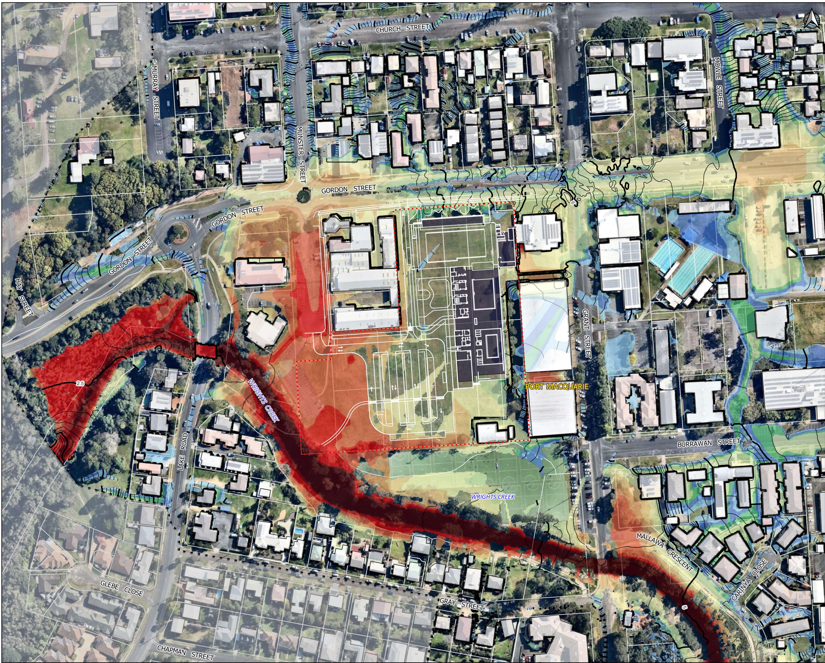
Figure C6 [A] Developed Case 1 in 200 AEP Flood Depth and Elevation Envelope of Local and Regional Flood Events
