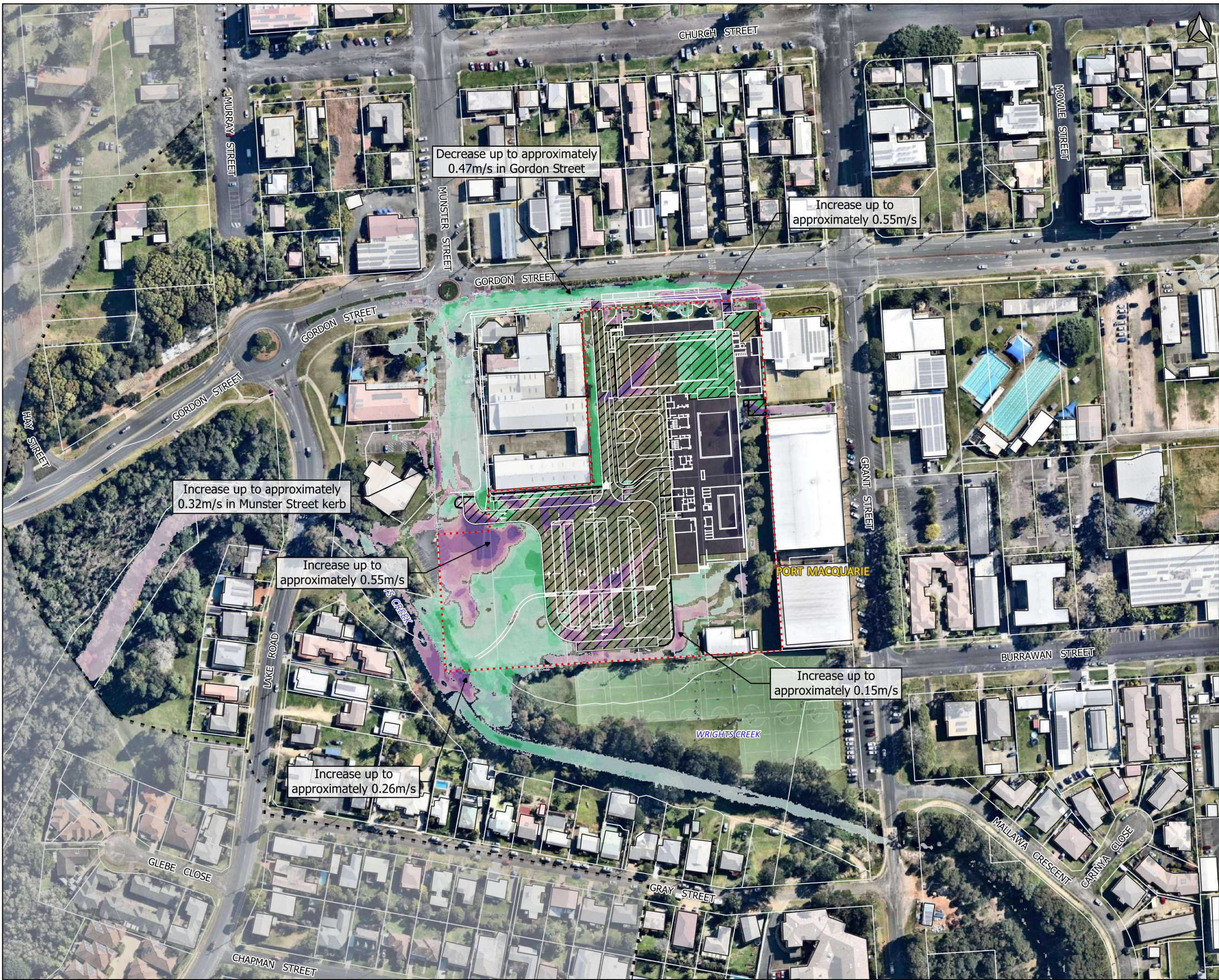
Figure D4 [A] Pre to Post Comparison 5% AEP Flood Velocity Local Catchment w/ Neap Tide Tailwater
