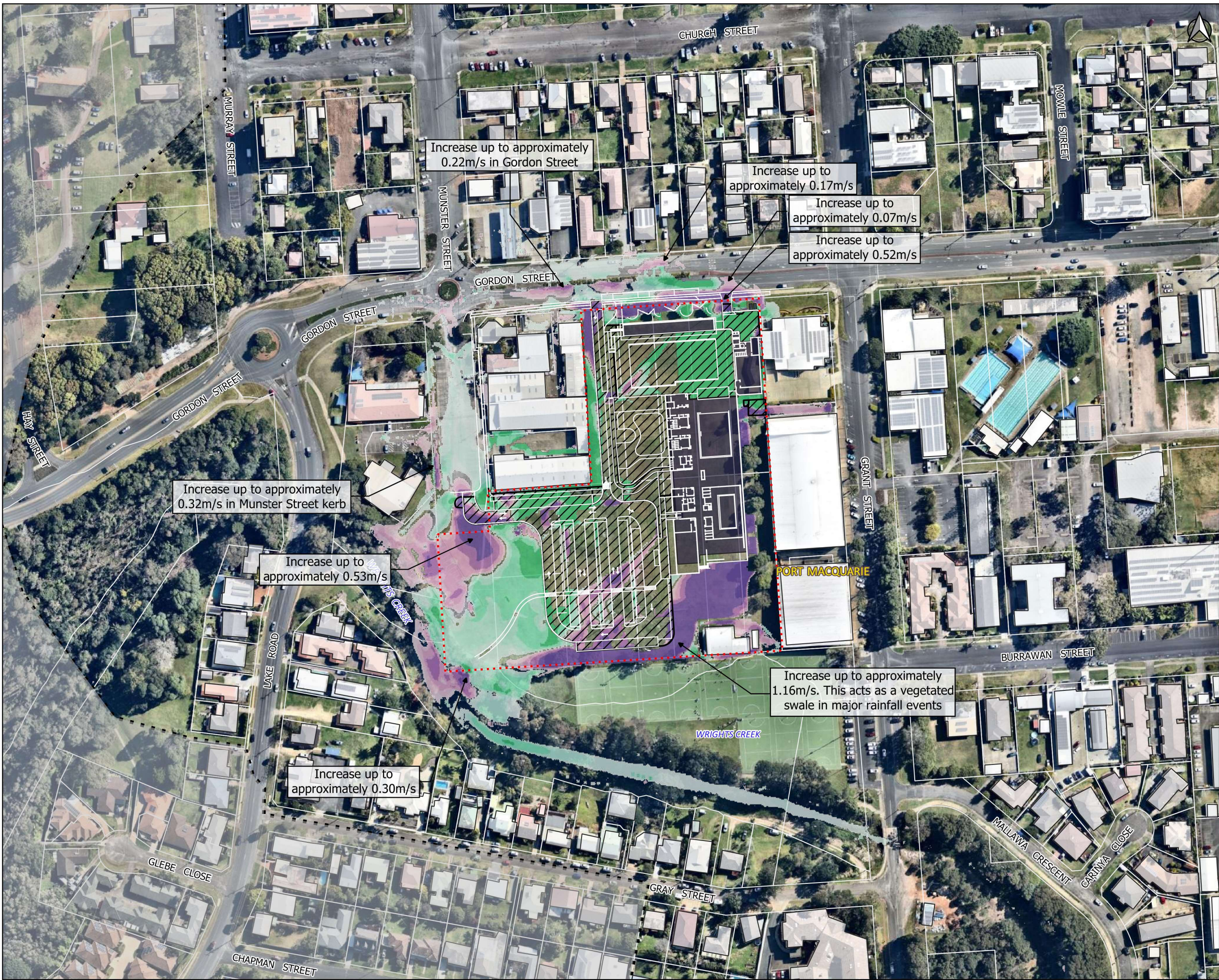
Figure D8 [A] Pre to Post Comparison 1 in 200 AEP Flood Velocity Local Catchment w/ Neap Tide Tailwater
